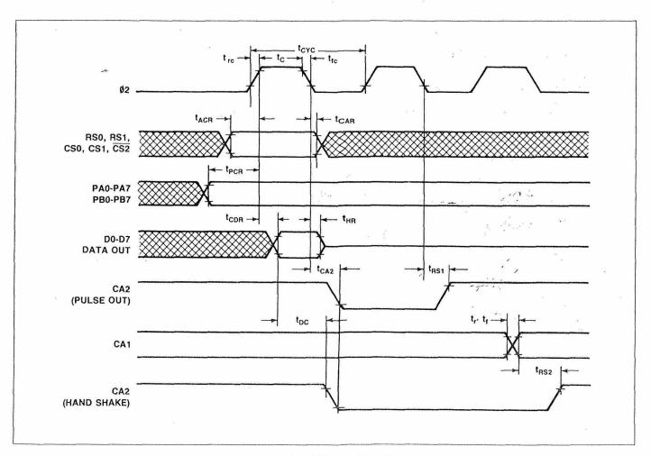
Figure 5. Read Timing Waveforms
