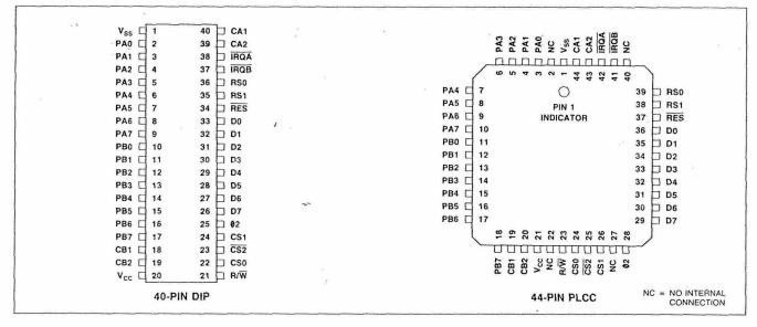
Figure 1. R65C21 Pin Assignments
